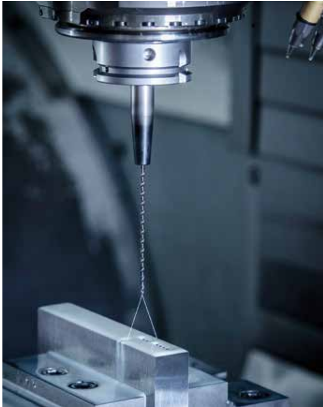
Ceratizit's WTX-Micro drills feature through-coolant and deliver tight-tolerance holes down to 0.8 mm diameter at depths up to 30xD. (Provided by Ceratizit)
