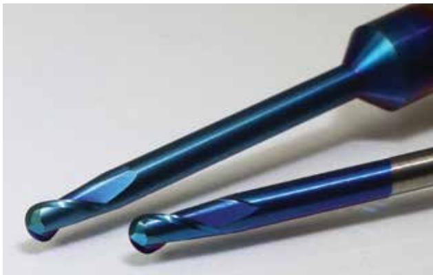
Mastercut Tool Corp.'s PowerN Coating (nACo) nano-composite (nc-AlTiN)/(a-Si 3 N 4 ) is designed for superalloys, hard material machining and high-heat applications (Provided by Mastercut)
